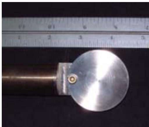
Figure 13. Photograph of the probe end of the 10-foot long disk impaction probe used to collect particle samples from the boiler flow. The stainless steel sampling disk is 1.85 inches in diameter.
