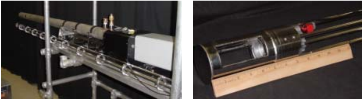
Figure 8. Photographs of the LIBS probe developed for boiler measurements. The photo on the left shows the complete optical probe assembly, alongside the YAG laser and water jacket assembly in which the probe fits. The photo on the right shows a close-up of the probe end, which has local water cooling, a laser focusing lens, and fiber-optic light collection for sparks produced in the center of the slotted flow-through section.
