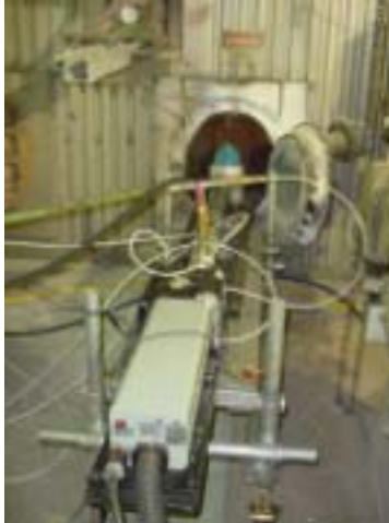
Figure 31. Photograph of the LIBS probe inserted into a maintenance beam port at Courtland.
